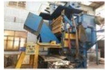
Automated Shot Blast
